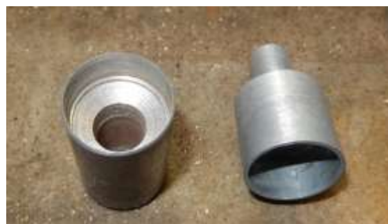
ABOVE: More vital pieces. The item on the left is a home made hole punch that will cut out 24mm diam discs of sandpaper. You then stick these discs of sandpaper onto the face of the cork. The item on the right is the cork holder. Its ID is a shade under 24mm, thus making the cork a snug fit up in it. The holder then mounts in the chuck of your drill press.
