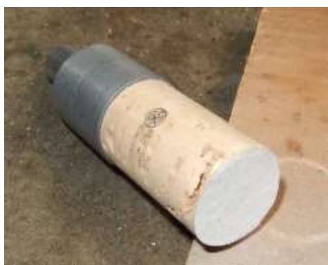
RIGHT: Before tackling the main job, it is advisable to experiment on a scrap piece of aluminium. I tried different grades of paper – 120, 240, 360 and 600.
