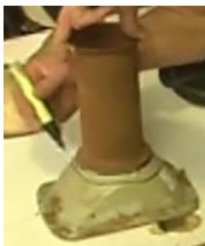
4 Using something suitably round, mark a circle on the donor reflector.
