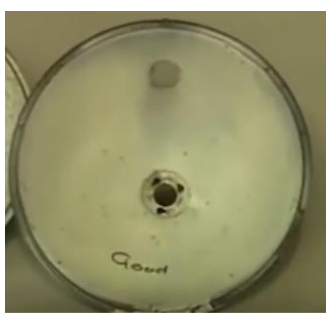
1 A typical vintage reflector that takes the standard bayonet type bulb.
