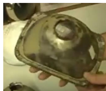
3 Your donor light will look like this once you've removed the bulb and its associated holding clips.
