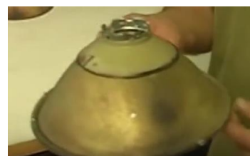
6 The freshly cut bulb holder can now be trial fitted on the top of the vintage reflector. The rest of the donor headlight set up can be thrown away.
