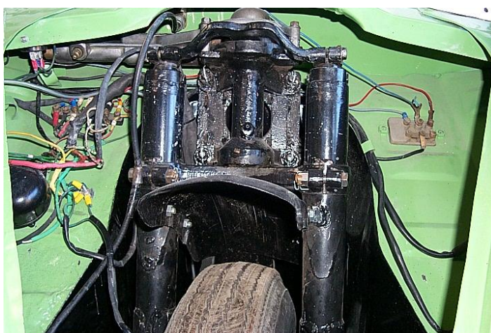
Under the 'bonnet'. Rack & pinion steering to the front fork
