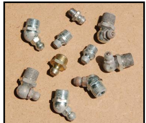
An assortment of modern grease fittings that is nearly identical to those patented by Joe Bystricky in 1934.
