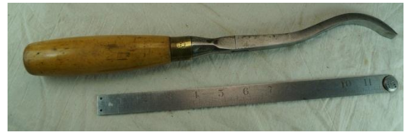
An early lock chisel with 12" ruler below for scale
