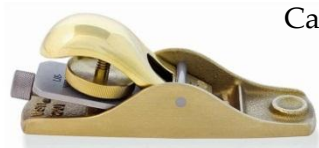
A low angle block plane
