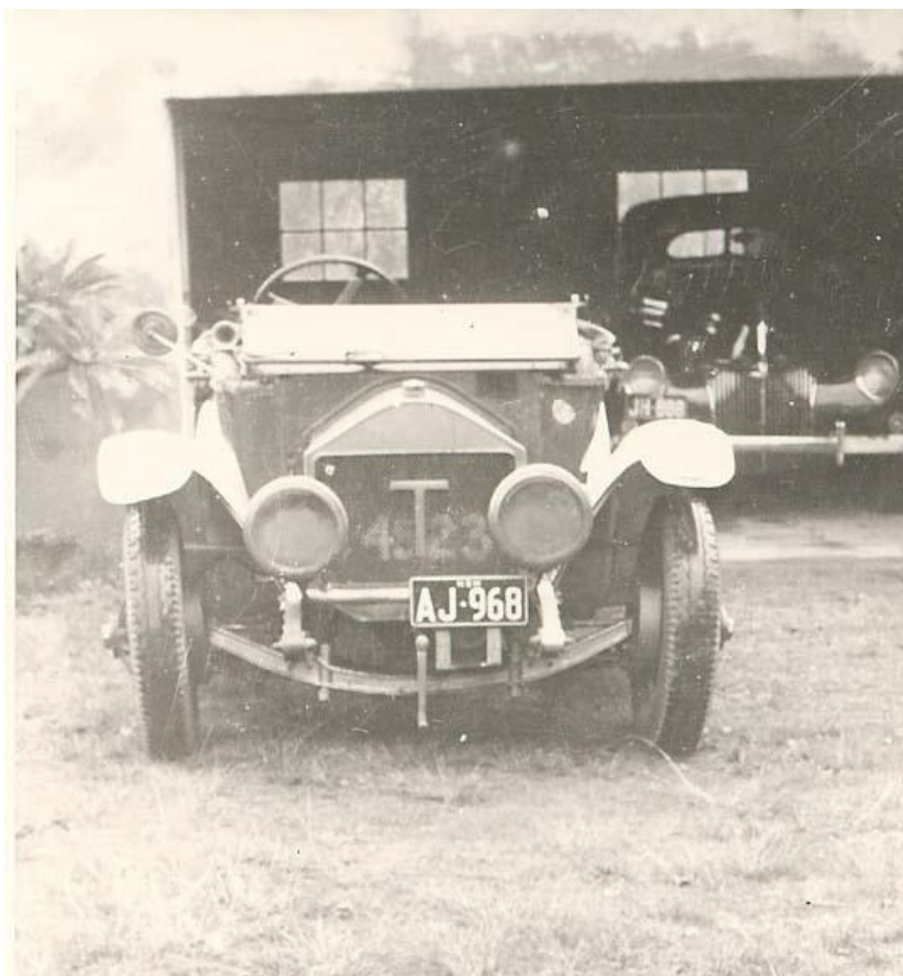
The original registration was 4523. Note the huge steering wheel, from a prewar bus, necessary to lighten the steering once the small 18 inch wheels were fitted.
