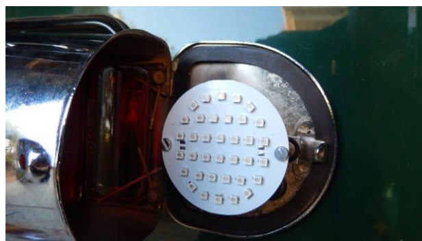
The bulbs now replaced with the lightboard. There are 36 red SMD's on this one. They all shine with one intensity for the taillight function, and go brighter still when the brake is applied. Not visible here are two white LEDs mounted at the rear of the board that stand off the board at 90° so they can shine across the number plate.
