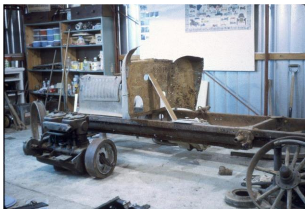
The assembled parts. Chassis now straightened by former member, Ross Millard, who owned a panel beating shop in Fyshwick.
