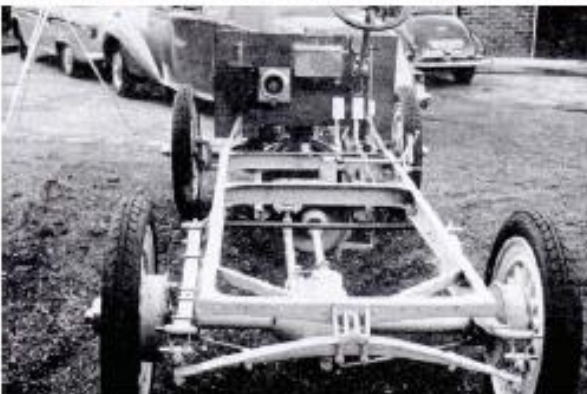
below left & right: Two views of 30 hp chassis No. 26355 left: Showing rear transverse and side spring mountings and shackle pins, dash board with trembler coil, ignition timer and distributor, and lubricator box. right: showing chassis frame bracing and attachments for rear suspension, rear-axle torque strut, thrust and braking links and the transmission-brake anchorage.
