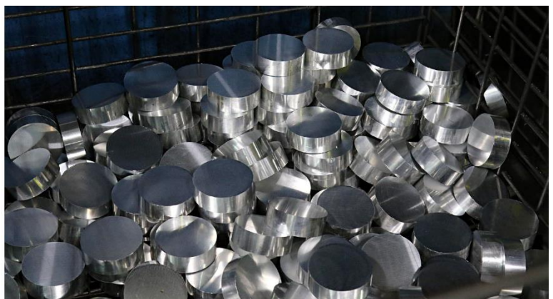
A stack of aluminium blanks ready for forging. They will be heated to 800°F in the forge and subjected to 18,000 tons of pressure to form their new shape.
